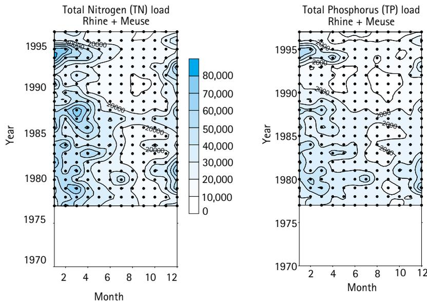
Figure 4.9: Comparison of the Total Nitrogen (TN) and Total Phosphorus (TP) load (tonnes/month) via Rhine and Meuse (Maassluis and Haringvliet).
