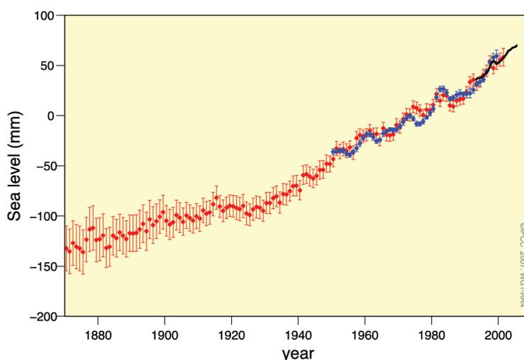
Figure 2: Annual averages of the global mean sea level based on reconstructed sea level fields since 1870 (red), tide gauge measurements since 1950 (blue) and satellite altimetry since 1992 (black). Units are in mm relative to the average for 1961 to 1990. Error bars are 90% confidence intervals. (Source: Solomon et al., 2007)
