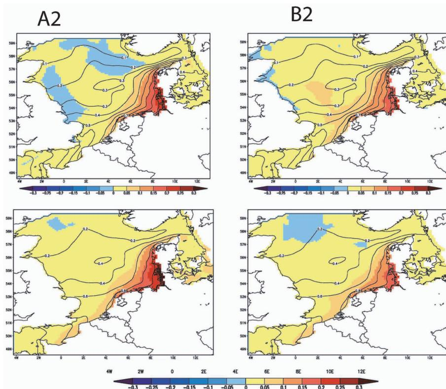
Figure 4: Changes in storm-induced water levels, calculated for IPCC A2 and B2 scenarios (columns) with two different models (rows). Isolines: current levels. Colours: calculated deviations from current levels (in m.). Source: Woth et al., 2006.
