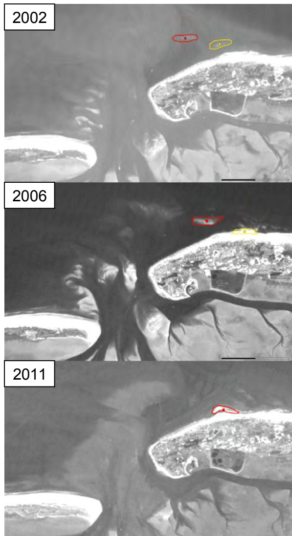
Figure 6.4.8: Landsat images of the ebb-tidal delta of Norderneyer Seegat, showing shoal attachment to the coast of Norderney in 2006 and 2011 (Ridderinkhof, 2016).
