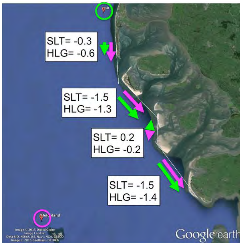
Figure 7.1.3: Littoral drift as determined on stations Helgoland (HLG) and Sylt (SLT) in 10^6 \text{ m}^3/\text{yr} (From: Ridderinkhof, 2016).
