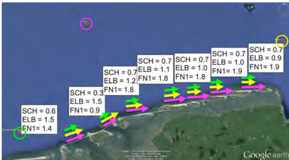
Figure 6.1.2: Littoral drift along the North Sea coast of Lower Saxony as determined on stations Schiermonnikoog (SCH), Elbe (ELB) and Fino1 (FN1) in 10^6 \text{ m}^3/\text{yr} (From: Ridderinkhof, 2016).
