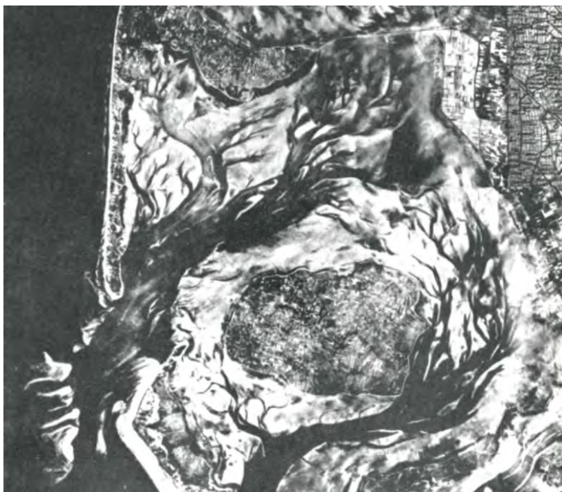
Figure 7.5.4: Hornum Tief in summer 1955. Extensive intertidal swash bars at the Northsea side of the ebb-tidal are still visible in 1955, which are largely absent in 2015, indicating that the changes took place after 1955.
