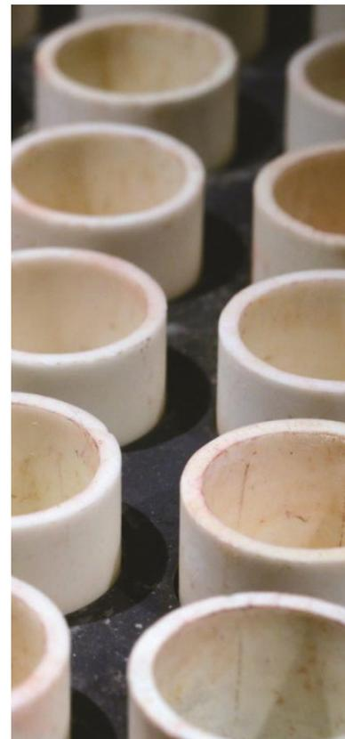
Crucibles aligned for determination of ash free dry mass of macrozoobenthos © Jan Drent
