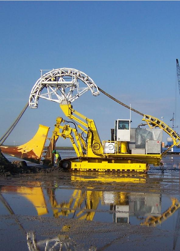
The vibration cable plough is a laying tool utilized for tidal flats
